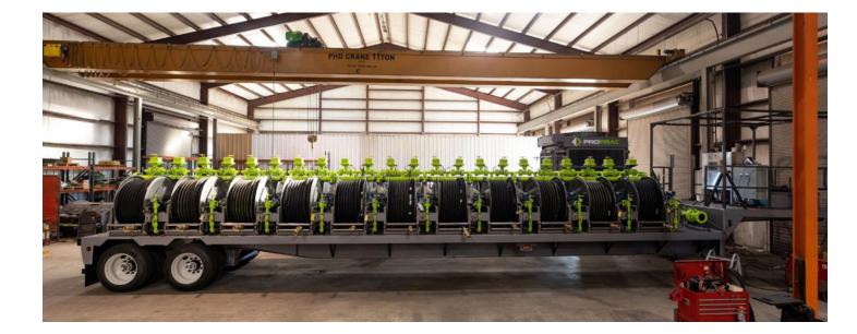
ProFrac's Gas Distribution Trailer optimizes flow rates and distribution rates to the frac pumps. Each valve has a real-time flow rate meter visible near each hose on the trailer. **These flow rates can be monitored from a live feed via the app at any time.**
